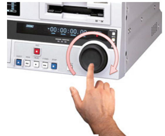
Figure 2. Use of the jog dial of a VTR
